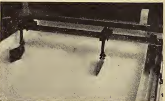
Here is shown the early formation of a wave at a discontinuity in the surface.
